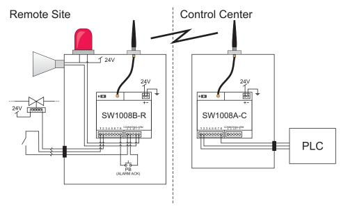
With this setup the PLC is able to control the valve and detect when the switch is opened or closed. Additionally when the switch becomes open it will sound an alarm horn and turns on a warning light. The push button will clear the alarm and signal the PLC.
